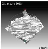
Kinect surface scans were aligned by picking pairs of points in each scan in Meshlab and running an ICP algorithm. This results in surfaces that capture all the metre-scale relief of this sample plot of penitentes.
