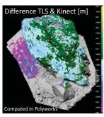
While the long range terrestrial laser scanner (TLS) can cover a much larger area, it is restricted by its viewing angle and even scanning from a vantage point onto snow penitentes in a stream bed, the Kinect has the advantage of mobility which enables the whole surface to be scanned.
